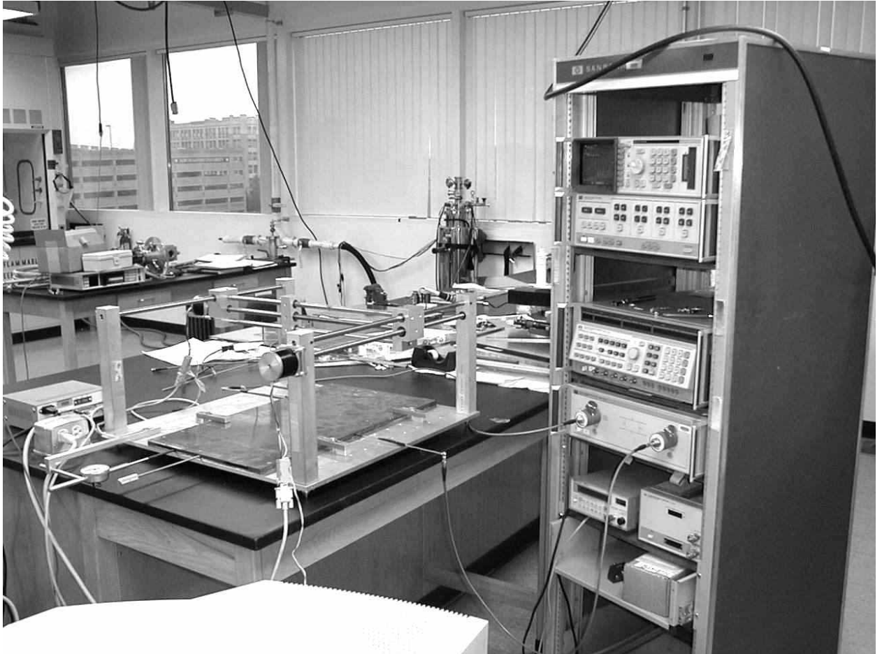
Figure 1: Photograph of the experimental setup at Northeastern for studying quantum chaos in microwave systems
