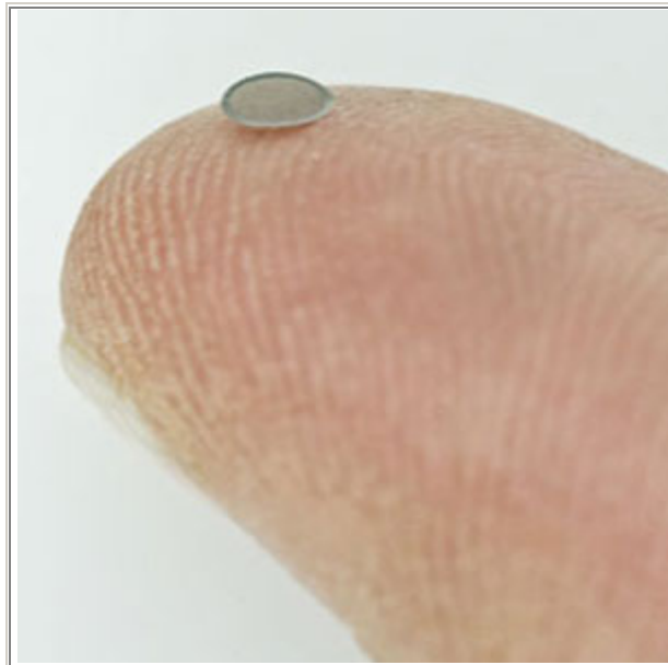
FIGURE 2. Kareem Elsayad and Katrin Heinze are working on a superlens that would be smaller than a contact lens, and the usable part would be even smaller, just a 0.25 millimeter square. (Image courtesy of Kareem Elsayad.)
